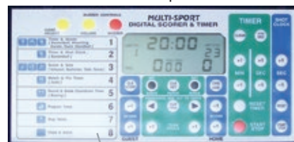
Digital display control panel on back for operator
